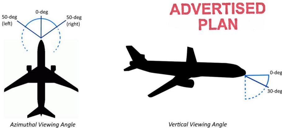
Figure 9. Diagrammatic illustration of Pilot's field of view (FOV) parameters (source: Forgesolar).
