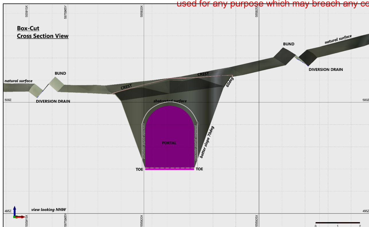
Figure 4.1d Box-Cut Cross Section View
