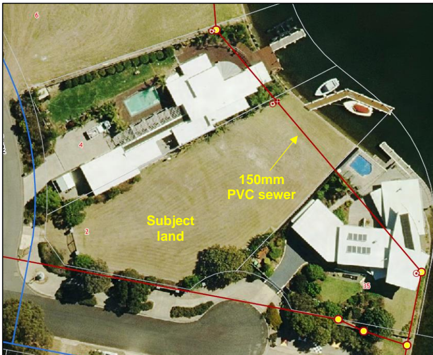
East Gippsland Water plans showing the sewerage infrastructure in the eastern part of the subject land (Source: EGW)
