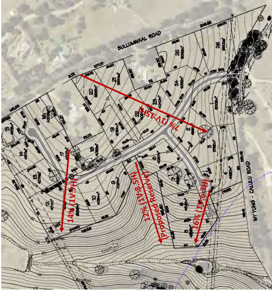
Figure 7: Indicative Site Slope and Direction of Fall
