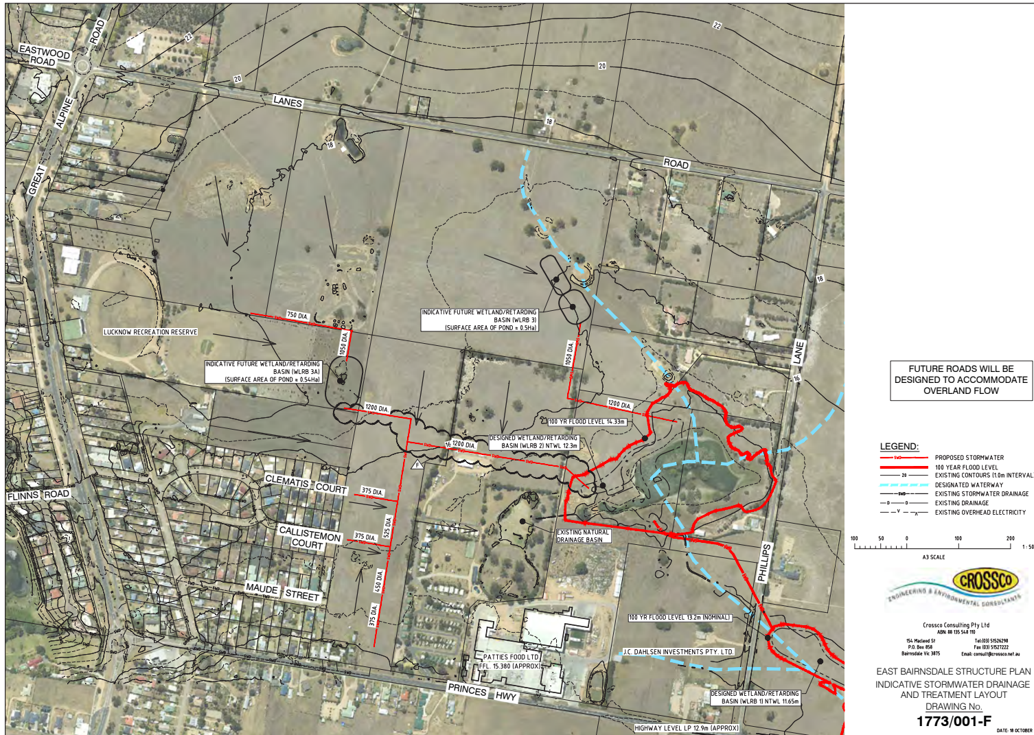
FIG 5o DRAINAGE INFRASTRUCTURE CONCEPT - NORTH
