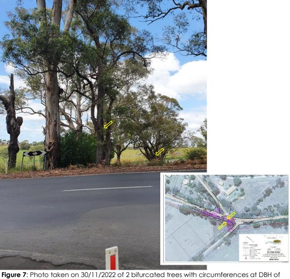
Figure 7: Photo taken on 30/11/2022 of 2 biturcated trees with circumferences at DBH of 157cm & 125cm that are proposed to be removed, with their locations shown on the inset plan
