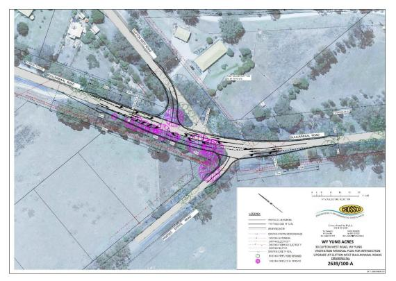
**Figure 2**: Vegetation Removal Plan for intersection works at Bullumwaal & Clifton West Roads
