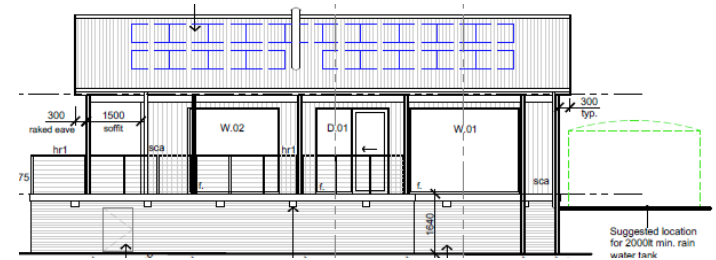
Figure 3 – North elevation – Sands Building Design
