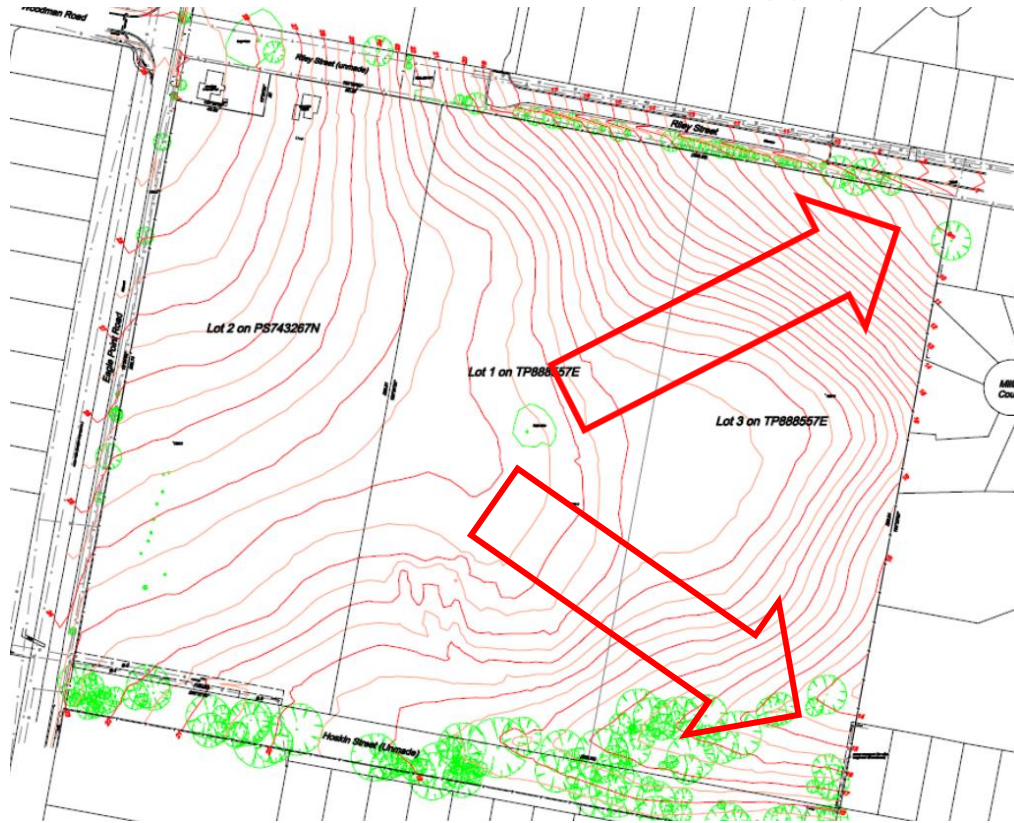
Extract from Feature and Contour Plan with arrows indicating direction of fall (Source: Freeman Land Surveying)
