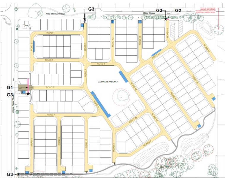
Visitor parking spaces shown in blue (Source: HLA, Dwg No. DA-03 Rev A)
