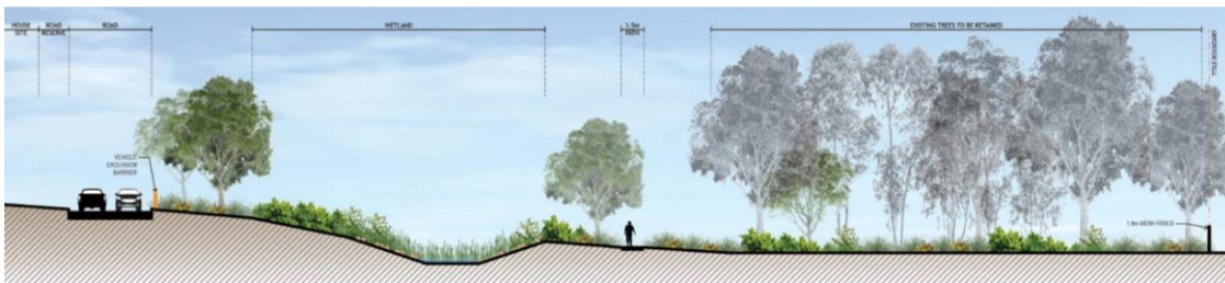
Drainage cross-section, depicting proposed improvements to the waterway (Source: HLA, Dwg No. DA-14 C Rev C)
