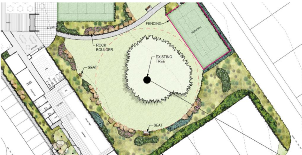
Extract from Clubhouse Landscape Plan showing TPZ as a red dashed line (Source: HLA, Dwg No. DA-08 A Rev A)
