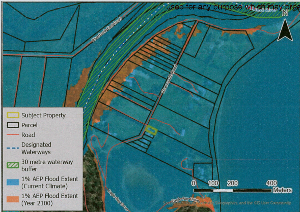
Figure 1 – Designated waterways and 1% AEP flood extent
