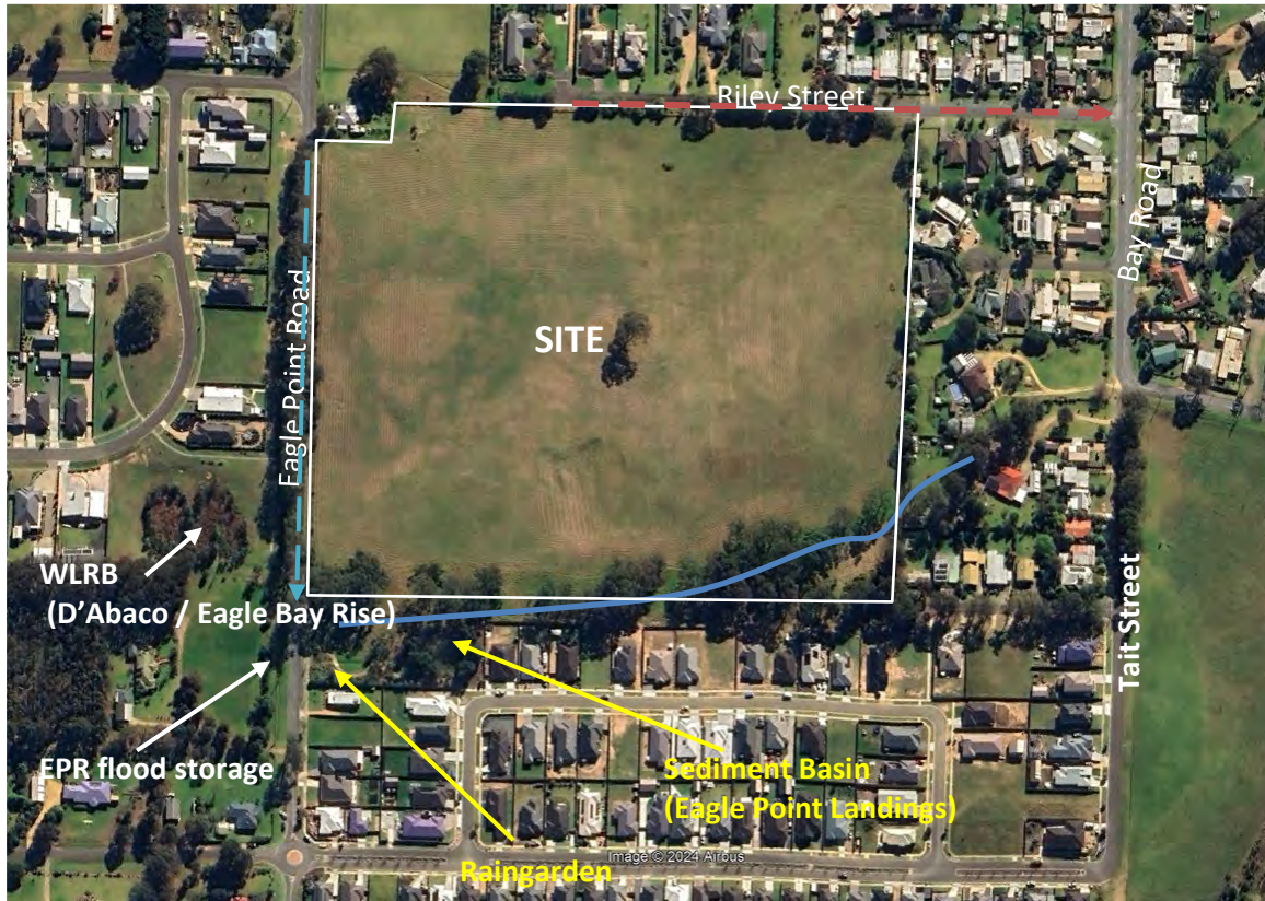
Figure 9: Existing Stormwater Infrastructure
