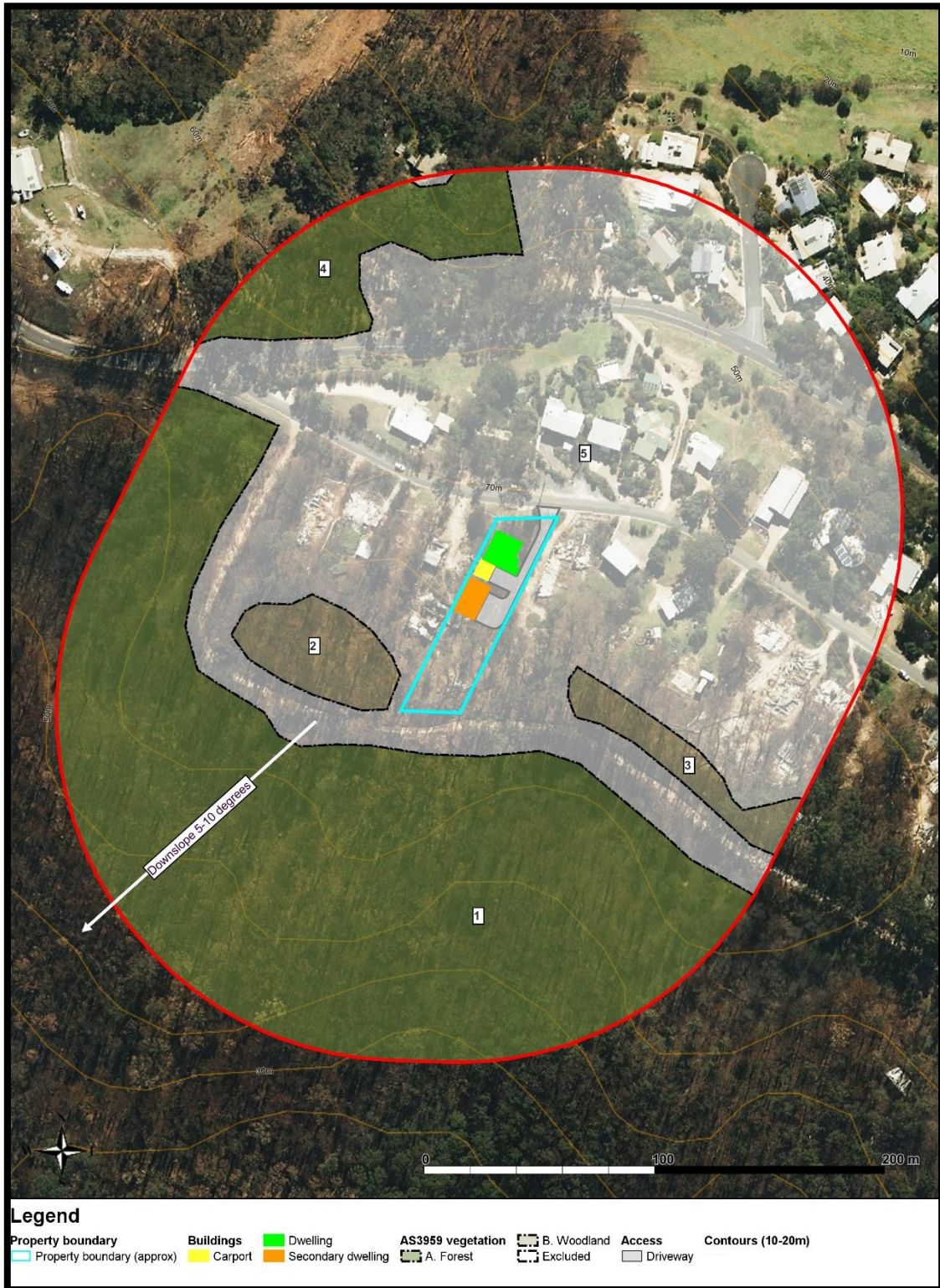
Figure 6 - Bushfire Site Hazard Assessment
