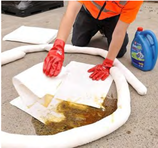
Figure 7.4. Containment and cleanup of a spill.
